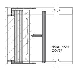
Adjust screen to line up to the edge of the cavity by loosening screw (A). Once lined up fix screws (A) and (B) into the bracket to lock it off.
