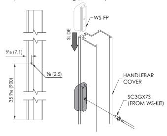
Before fitting handlebar cover (assembly as per screen instructions) ensure the cords are not twisted or tangled.
