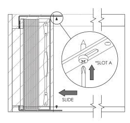
Pre-drill  $V_8$  (2.5) hole in handler bar cover (as shown below). Slide finger pull into t-slot and screw fix into place. Fit remaining parts as per INSTSCREEN
