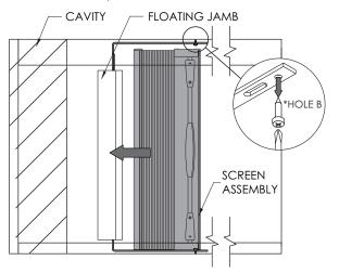
Push assembly into the cavity (Ensure screen is level). Screw fix brackets into place. Continue with screen installation as per INSTSCREEN.
